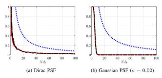
Figure 1. Empirical realization of the quantities  $\|S - E_1 I_K\|$  (in red/solid),  $\|M - E_1 I_K\|$  (in black/dash-dot), and of theoretical upper bound Equation (14) from Lemma IV.1 (in blue/dotted), for varying  $\Delta$ . Herein, N = 501.
