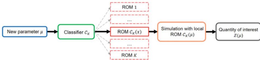
Fig. 2.5 Exploitation phase of a dictionary-based ROM-net. K local ROMs, combined with a classifier C_K for automatic ROM C_K(\mu) recommendation, are used to predict the quantity of interest Z(\mu)
