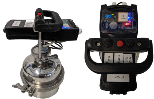
Figure 5. Side view of the assembled chamber positioned on the collar and top view of the chamber.
