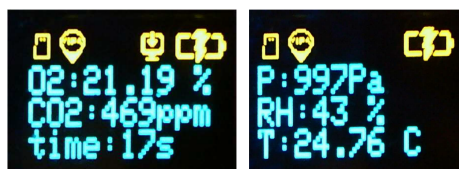
Figure 2. Small (0.96 in.), yet very readable, OLED display permuting screens with different useful information.
