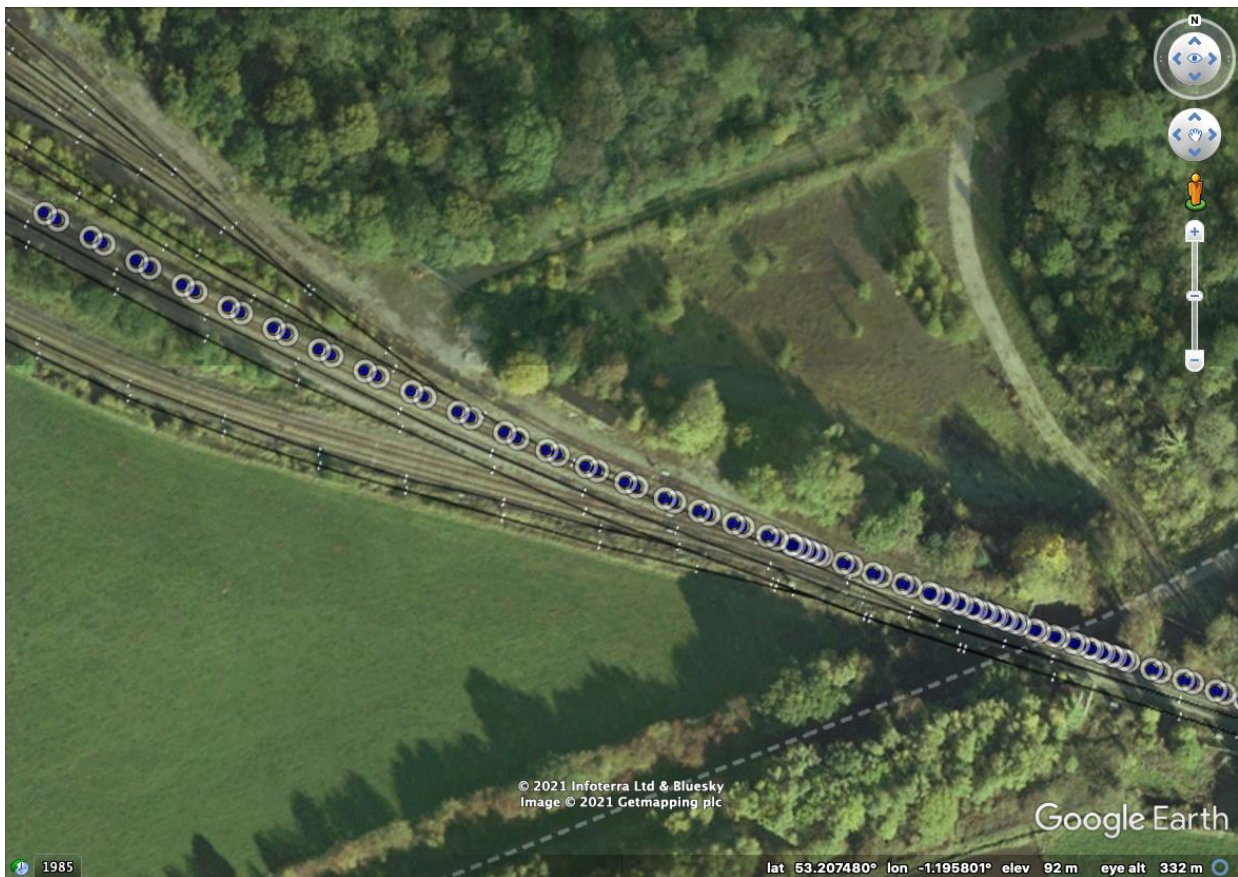
Figure 12. Demonstration of the simulation phase of the GLS simulator. White circles are input values provided by RSS and blue dots are the corresponding simulation delivered by GLS. This case corresponds to the ideal case, without no feared events.
