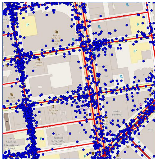
Figure 3: Example of inaccurate GNSS locations (in blue) from the CabSpotting Project in San Francisco (USA). In Red the underlying road network from OpenStreetMap
