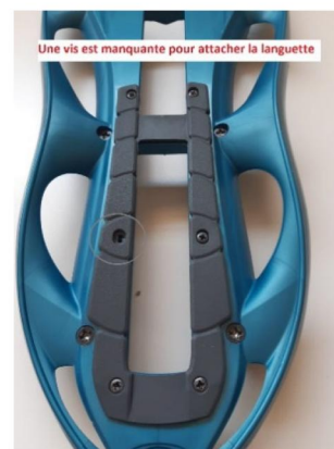
Error 6: Missing a screw
