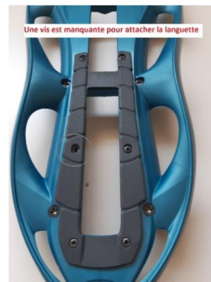
Error 6: Missing a screw
