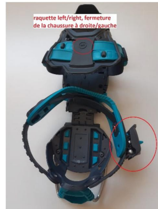
Error 2: Fastener on wrong side
