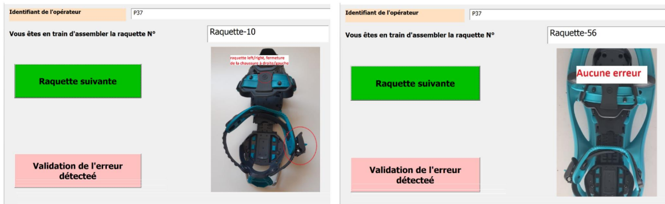
Figure 6. AIEDS when error is detected (left) and no error detected (right).
