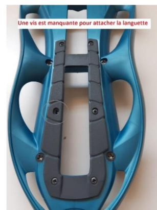
Error 6: Missing a screw
