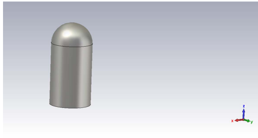
Figure 15. The simulated PEC cylinder with a hemispherical end oriented along z axis.
