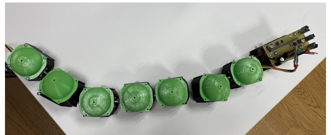
Fig. 3. Picture of the snake robot with the locomotive and 7 wagons. Wires linking the locomotive to wagons are know shown.
