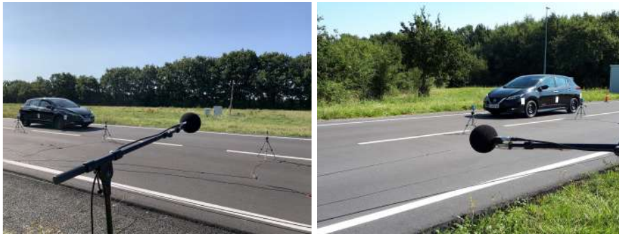
Figure 5.2: Location of the microphone at 7.5 m relatively to the tested track: prototype test section P (left), prototype test section PCR (right).
