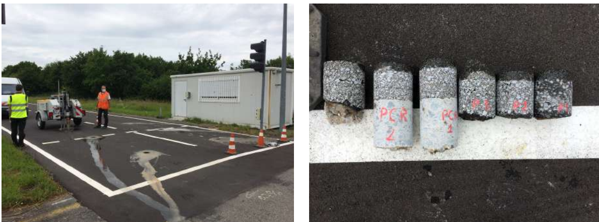
Figure 3.15: Drilling of core samples in the prototype (left) and picture of the six core samples (right).
