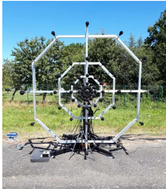
Figure 2.11: Setup of the 61-microphone plane array.
