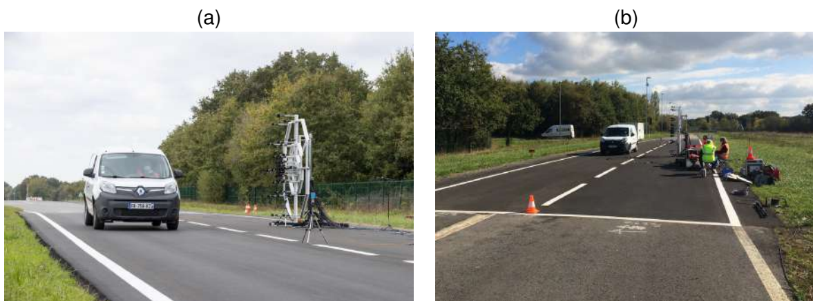
Figure 4.17: Pictures of the simultaneous CPB and microphone array tests on the prototype test sections P (a) and PCR (b) in the case of the Renault Kangoo ZE.
