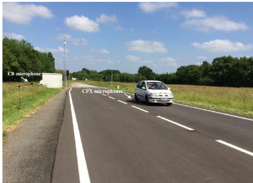
Figure 4.27: Simultaneous CPX and CB noise tests on prototype test section P ( E \rightarrow W direction).
