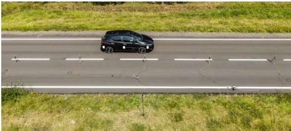
Figure 5.1: Setup of the experiment over the 20 m long test section of prototype road surface PCR.
