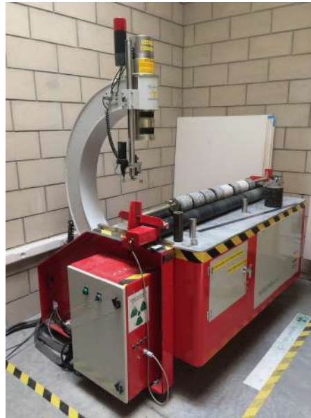
Figure 3.16: Gamma densimeter used to measure actual density and air-void content from the core samples drilled on the prototype test sections.
