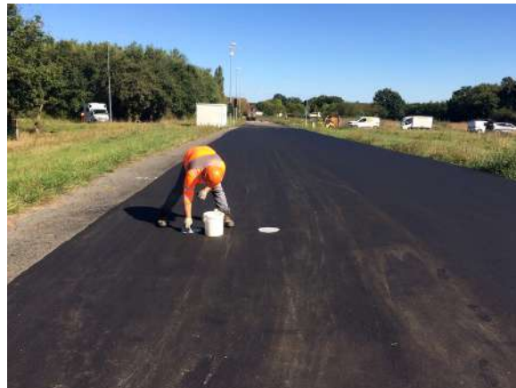
Figure 3.14: Sand patch MTD measurement by Colas on 8 September 2020.
