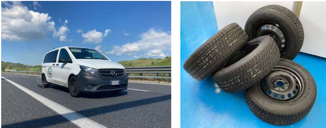
Figure 4.32: Test vehicle (left) and SRTT tyres (right) used by IPOOL for CPX measurements.
