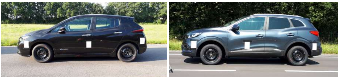
Figure 5.4: Nissan LEAF (left) and Renault KADJAR (right) fitted with one set of test tyres and three reflecting plates.
