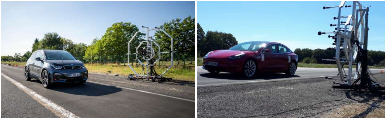
Figure 2.12: Microphone array and vehicle pass-by on road surface N – Left: overview with the BMW i3 – Right: reflecting plates on the Tesla Model 3.
