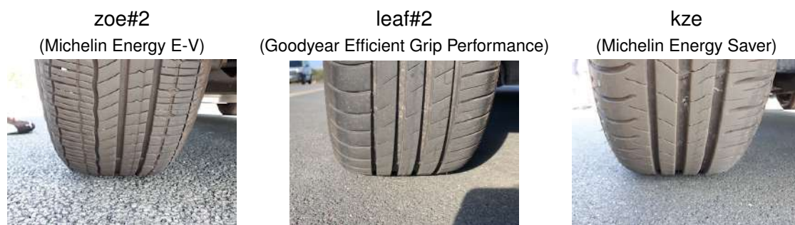
Figure 4.15: Tread pattern of the tyres fitted on the EVs tested within sub-action B2.3.
