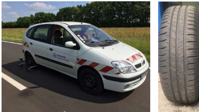
Figure 4.25: Test vehicle (left) and standard commercial tyre (right) used for simultaneous CB and CPX tyre/road noise measurements.
