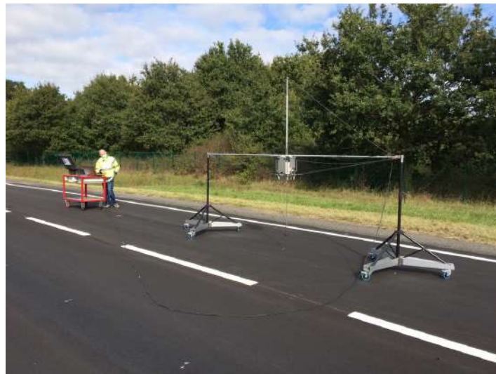
Figure 4.7: Sound absorption measurement on the prototype test section PCR in September 2020.
