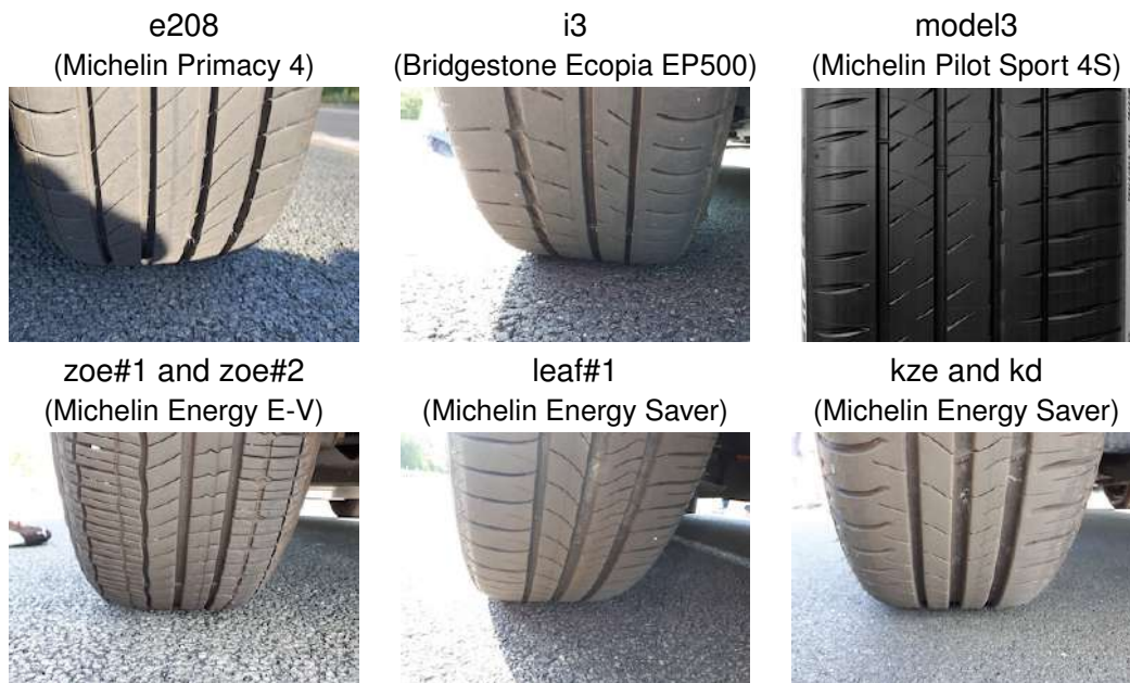
Figure 2.8: Pictures of the tread pattern of the tyres fitted on the test vehicles.
