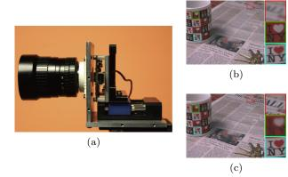
Fig. 18: The camera with a flexible depth of field prototype (a), a scene captured with a conventional camera (b), the same scene captured with a plane of sharp focus tilted by 53° (c). Reproduced from (Kuthirummal and Nayar 2007).
