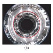
Fig. 23: The *cata-fisheye camera* prototype (a) and an image it acquires, made of two rings (the one with red border is captured by the mirror, the rest by a fisheye lens) (b). Reproduced from (Krishnan and Nayar 2008).
