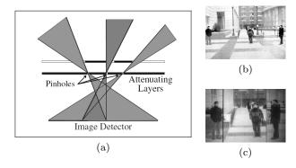
Fig. 5: A lensless camera with 3 pinholes (a), an image of a scene captured by a conventional camera (b) and the same image, taken at the same viewpoint, captured with the lensless camera configured as Fig.5a (c) (reproduced from (Zomet and Nayar 2006)).
