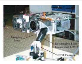
Fig. 27: The *Programmable imaging* prototype (reproduced from (Nayar et al. 2006))
