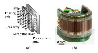
Fig. 11: (a) TOMBO architecture (reproduced from (Chan et al. 2006)), (b) CurvACE prototype (reproduced from (Floreano et al. 2013)).
