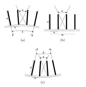
Fig. 8: The light rays captured for a concave (a), planar (b) and convex (c) curvature of the Söller Collimator. Reproduced from (Koppelhuber and Bimber 2017).
