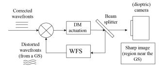
Fig. 28: Adaptive Optics with a Deformable Mirror (simplified) principle.
