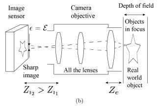
Fig. 13: The objects are within the depth of field  $\delta$  far from the camera if  $Z_i$  is close to f (a). Extending  $Z_i$  by a focusing extension  $Z_e$  allows to image near objects (b).
