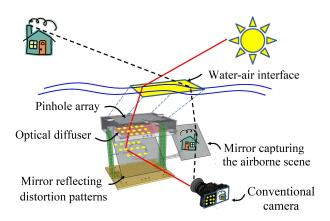
Fig. 24: Stellar Maris working principle (c) (reproduced from (Alterman et al. 2014)).
