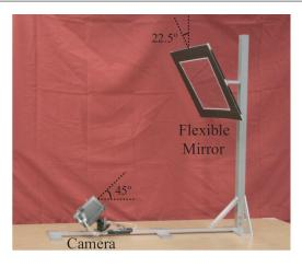
Fig. 26: The flexible mirror imaging prototype. Reproduced from (Kuthirummal and Nayar 2007).
