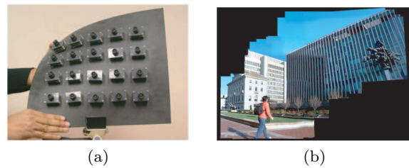
Fig. 31: The Flexible Camera Array prototype, flexed, (a) and the image acquired, stitched by the scene collage algorithm (b) (reproduced from (Nomura et al. 2007)).
