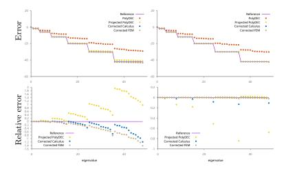
Fig. 6: Smallest 49 eigenvalues of the Laplacian on unit sphere with discretization step 0.1 (left) and 0.01 (right). Relative error is given by  $\hat{\lambda} - \lambda$ , where  $\hat{\lambda}$  is the approximated eigenvalue and  $\lambda$  the correct value.
