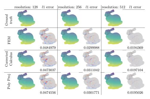
Fig. 7: Comparison between classical cotan Laplacian of a function defined on a triangle mesh and the digital Laplacian operators. All three operators have comparable performances. The error decreases as the resolution increases, suggesting that all three operators are convergent.
