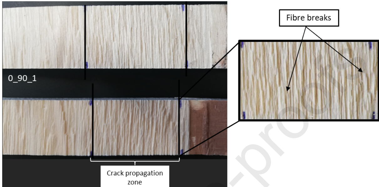
Figure 15. Fracture surfaces of a specimen with a 0^{\circ}/90^{\circ} interface.
