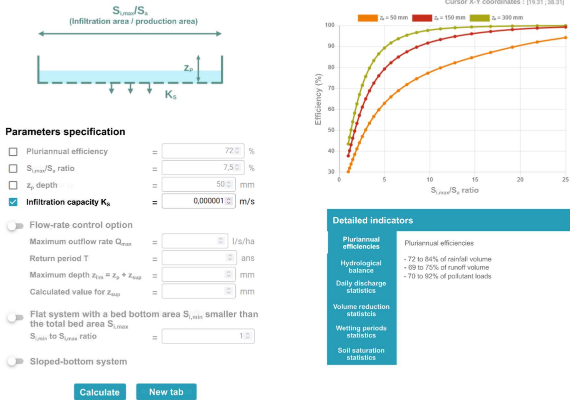
Figure 3 - Oasis-app interface (output screen for K_s = 10^{-6} m/s and after selection of the S_{i,max}/S_a = 7.5\% and z_p = 50 mm from the graphical panel). Translation from French for the main controls and menus.
