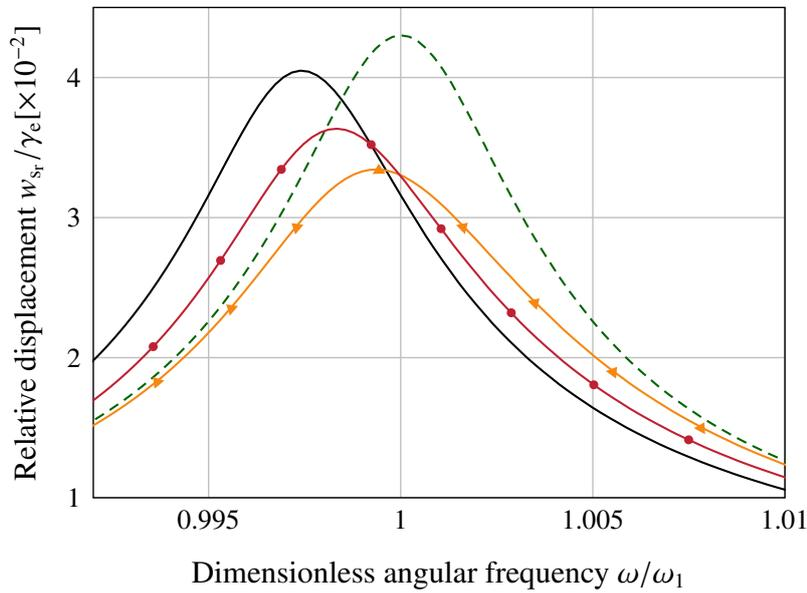
Figure 1: Relative displacement normalized by the base acceleration as a function of the dimensionless angular frequency: (---)  $\gamma_e = 0.1 \text{ mm s}^{-2}$ , (---)  $\gamma_e = 35 \text{ mm s}^{-2}$ , (—●—)  $\gamma_e = 135 \text{ mm s}^{-2}$  and (—)  $\gamma_e = 200 \text{ mm s}^{-2}$ .
