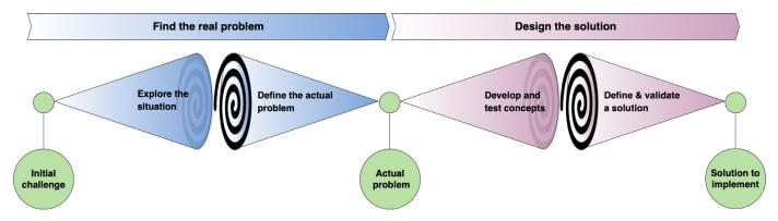
**Fig. 1.** A model of the design process. The 'double diamond' structure depicts how designers alternate between phases of divergent and convergent thinking to move from an ill-defined initial challenge to the actual problem that needs tackling, to a solution ready for implementation.<sup>3</sup> The 'spiral' patterns highlight how design projects move between steps in an iterative, non-linear way.<sup>55</sup>
