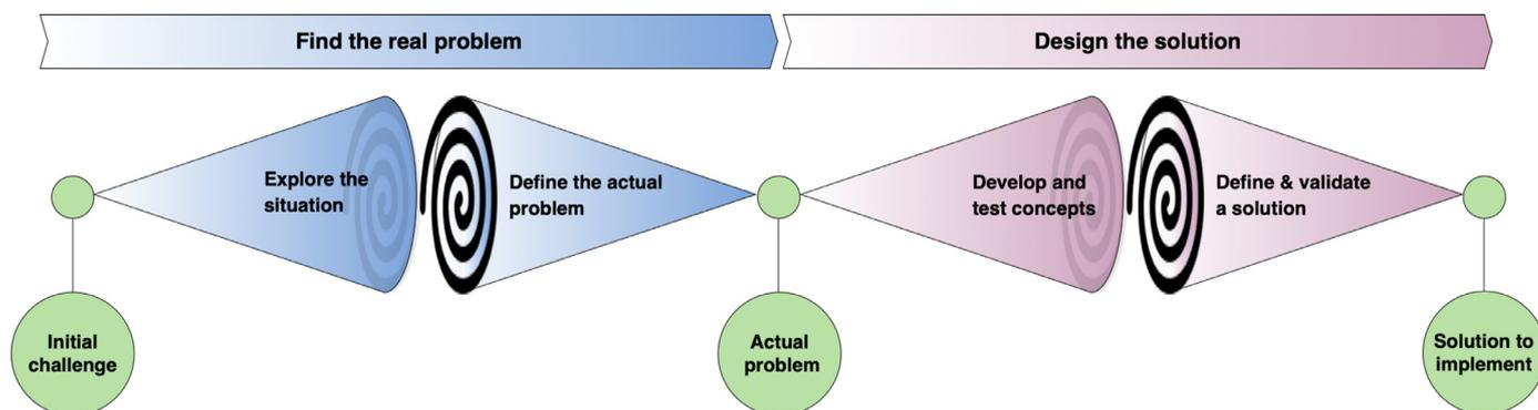
**Fig. 1.** A model of the design process. The 'double diamond' structure depicts how designers alternate between phases of divergent and convergent thinking to move from an ill-defined initial challenge to the actual problem that needs tackling, to a solution ready for implementation.<sup>3</sup> The 'spiral' patterns highlight how design projects move between steps in an iterative, non-linear way.<sup>55</sup>
