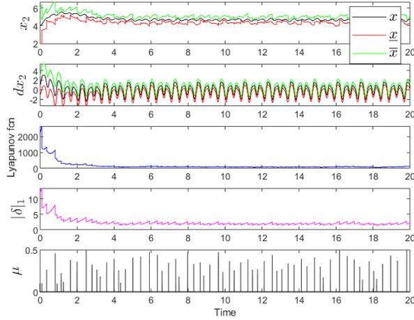
Fig. 2: The estimation bounds for the state variables  $x_2$  and  $\hat{x}_2$ , the Lyapunov function (26), the norm of estimation error width  $\delta = \bar{e} + e$ , and the inter-measurement time  $\mu \in [0.1, 0.5]$ .
