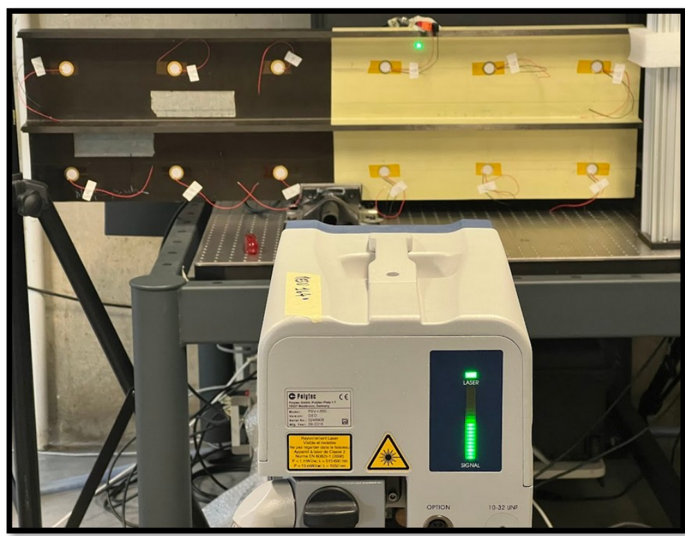
Stiffened composite panel with a curvature
