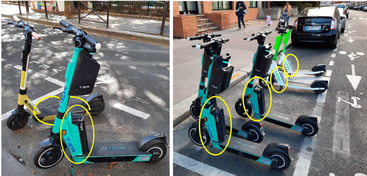
Fig. 1. Shared e-scooters in Paris streets: the adoption of swappable batteries
