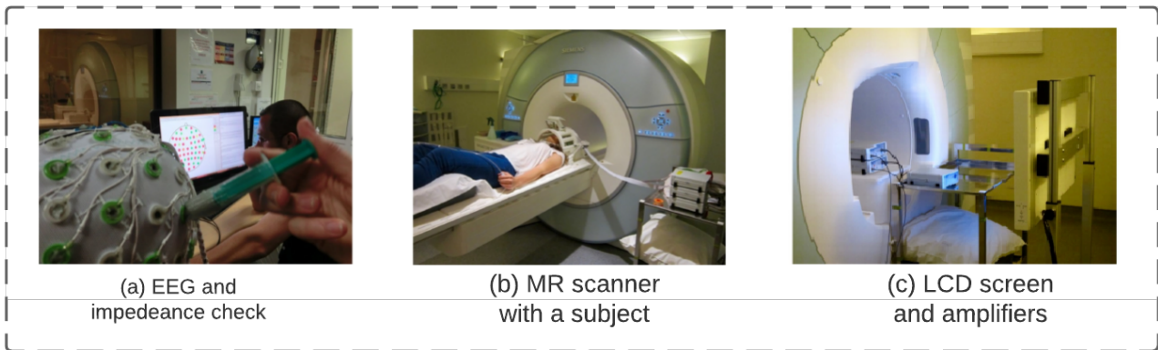
Figure 5. Photography of the preparation of a simultaneous EEG-fMRI-NF session with a 3T MRI and a 64 EEG cap. (a) EEG subsystem installation and impedance check outside the MR environment, (b) Installation of the MR coil and EEG impedance recheck, (c) Placement of the amplifiers, battery and LCD display.
