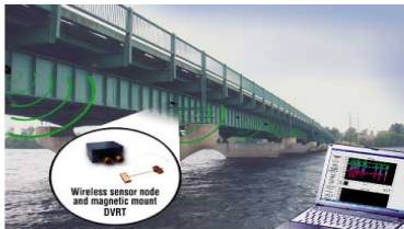
3. Wireless sensors are used to measure long-term stress and strain in civil engineering structures like buildings and bridges. (Courtesy: Microtrain Inc.)
