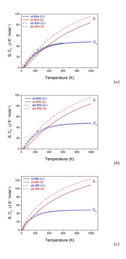
Figure 4. Heat capacity at constant volume  $(C_V)$  and entropy (S) of zinc-blende and qtz boron pnictides as functions of temperature: BAs (a), BSb (b) and BBi (c). Experimental heat capacity data for zb-BAs [2,52] are shown as gray symbols.
