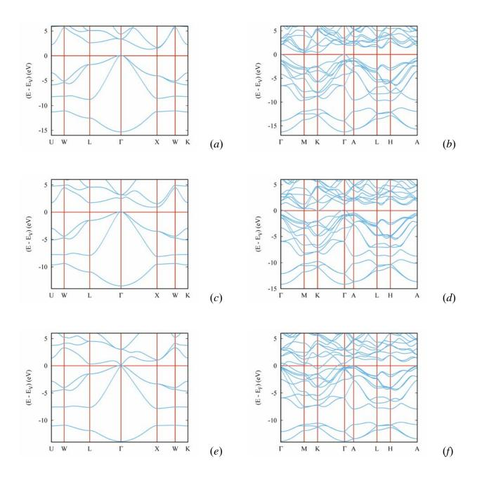
Figure 5. Electronic band structures of *zb*-BAs (*a*); **qtz** BAs (*b*); *zb*-BSb (*c*); **qtz** BSb (*d*); *zb*-BBi (*e*), and **qtz** BBi (*f*).
