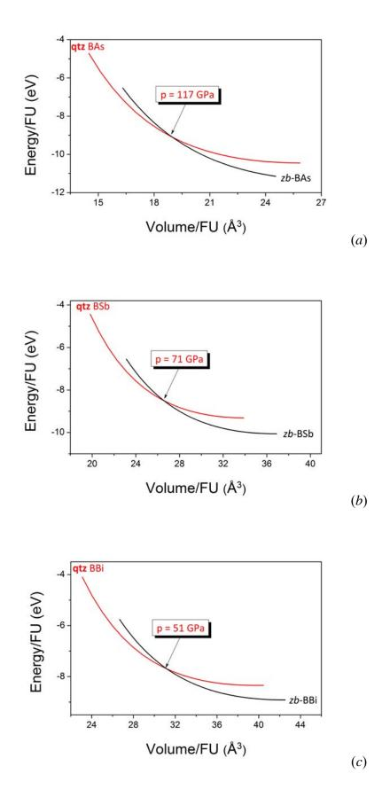
Figure 2. Calculated total energy per formula unit as a function of volume for zinc-blende and **qtz** boron pnictides: BAs (a), BSb (b), and BBi (c).
