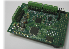
8 generic analog channels 24 bits / 50 kHz
