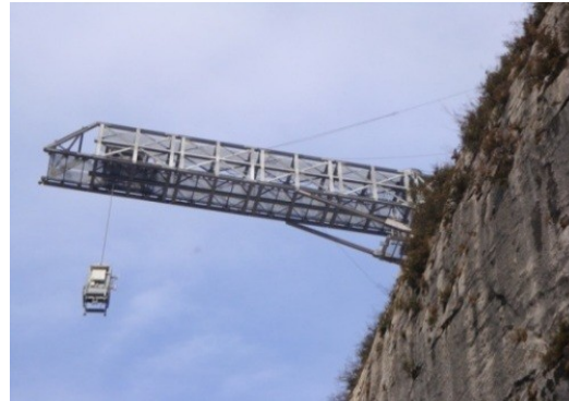
Facility for Impact assessment of rock fall (Up to : 20 t / 12 m)
