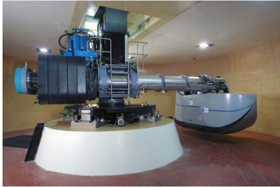
Geotechnical centrifuge : behaviour survey of geotechnical structures (foundations, off-shore anchorages, embankment, retaining structures) on a small-scale
