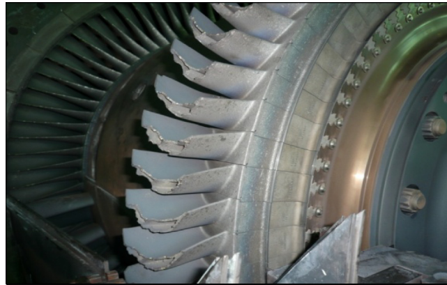
Fig. 2. Wear of the axial compressor fins.
