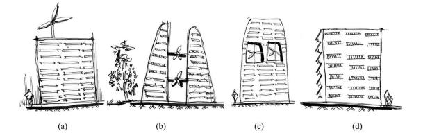
**Figure 2.** Different wind turbine systems : (a) on the roof, (b)between two buildings, (c) inside through-building openings, (d) into building's skin Source : Hassanli and al. 2017 [23]
