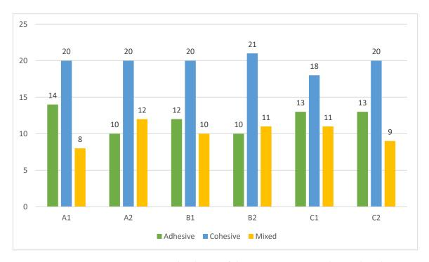
**Figure 3.** Frequency distribution of the 252 specimens according to the sub-groups and modes of failure.
