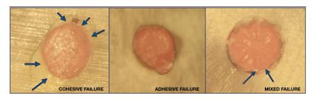
Figure 2. Samples under magnification  $\times 20$  as observed just after push-out test illustrating the three possible bond failures. The push out test stops automatically after decohesion of the gutta-percha cone. The latter is nevertheless still visible on the pictures due to its incomplete dislodgment. The blue arrows indicate some areas showing the sealer.
