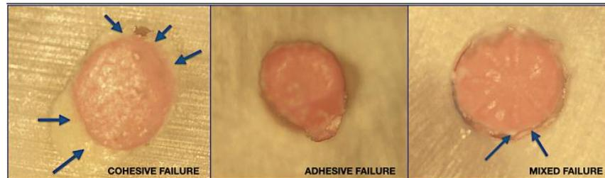
**Figure 2.** Samples under magnification ×20 as observed just after push-out test illustrating the three possible bond failures. The push out test stops automatically after decohesion of the gutta-percha cone. The latter is nevertheless still visible on the pictures due to its incomplete dislodgment. The blue arrows indicate some areas showing the sealer.
