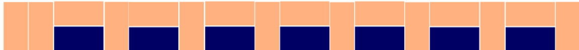
Figure 12: Top view of a pattern observed after a failure by overturning. The light color blocks remained stable and the dark color ones have fallen
