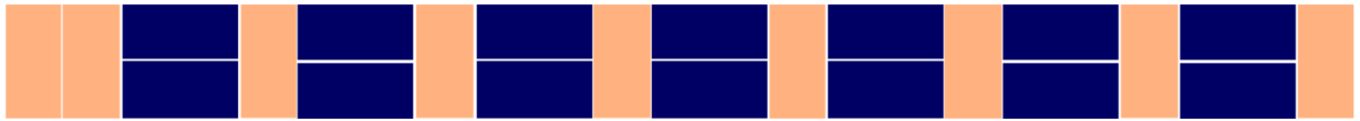
Figure 4: Top view of an assemblage studied in the experiments. Stretchers (light color) and headers (dark color) are presents
