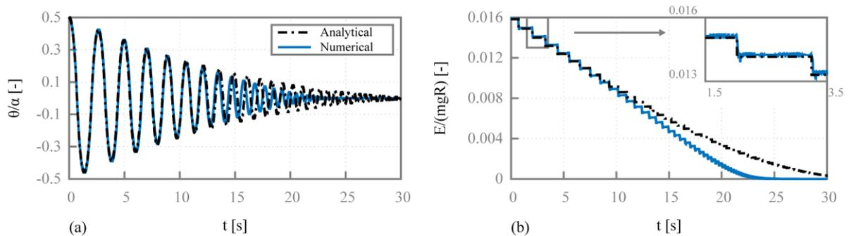
Figure 2: Behaviour of the viscous damping model. Comparison with the analytical model, in terms of variation of the (a) rocking angle and (b) total energy content over time. Details of the examined structure:  $2h = 4.2$  [m],
