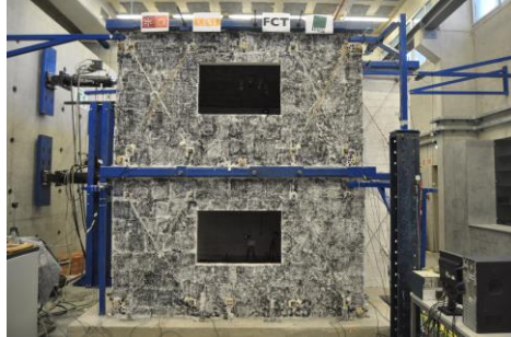
Figure 5. Building façade that DIC was applied
