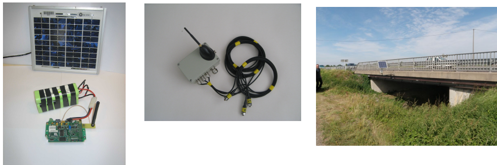
Figure 5: Power Management Board used with PEGASE WSN in a real SHM application
