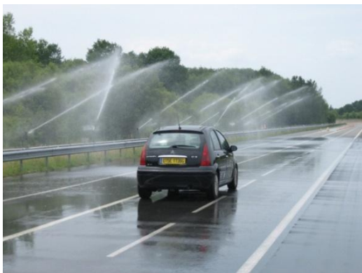
Fig. 3. Real-time Skid Resistance Prediction on Wet Road and Advisory Speed Computation on the Test Track of Ifsttar in Nantes.
