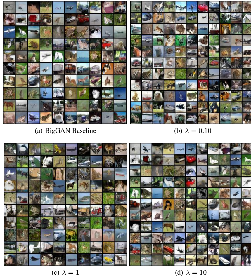
Figure D.15: CIFAR-10: Samples are drawn from different BigGAN trained on the PR-Divergence. We observe that when \lambda increases, the recall decreases going to a various range of colored images to mostly brown images.
