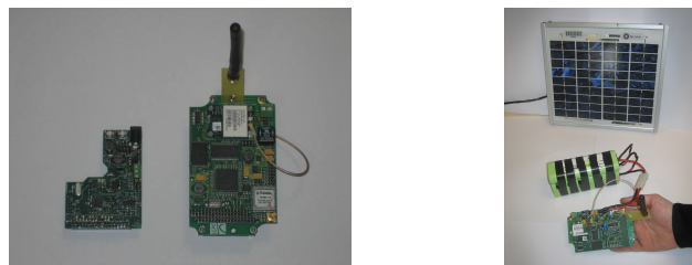
Figure 6: Physical implementation: a power manager daughter board
