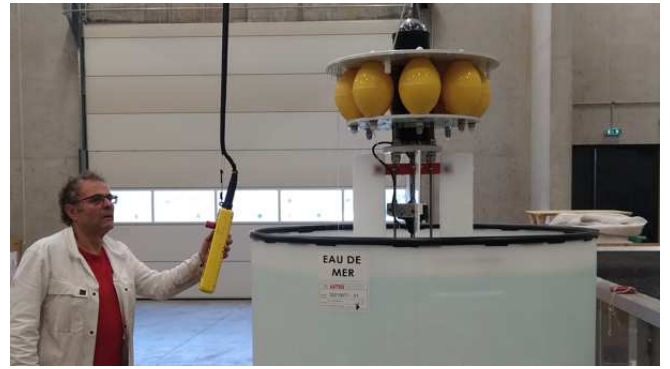
Fig.2. Ballasting the VVP at the SAM (Service Atmosphere et Mer) technical facility of the MIO (Mediterranean Institute of Oceanography)
