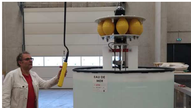
Fig.2. Ballasting the VVP at the SAM (Service Atmosphere et Mer) technical facility of the MIO (Mediterranean Institute of Oceanography)
