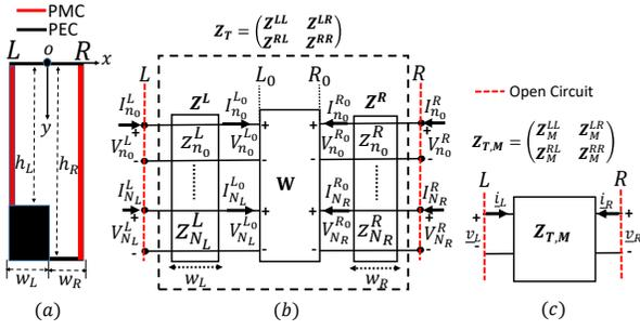
Fig. 2. (a) Schematic of the FSS-GRW waveguide cross-section with the dimensions  $w_L = \frac{d_x}{2}$ ,  $w_R = \frac{P_x - d_x}{2}$ ,  $h_L = \frac{P_y - d_y}{2}$  and  $h_R = \frac{P_y}{2}$ . (b) Corresponding GTR multi-modal network representation. (c) GTR network representation at the resonance frequency  $f = f_M$ .
