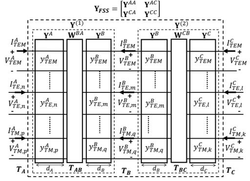
Fig. 3. Multi-port network representation in terms of the full FSS admittance matrix  $\mathbf{Y}_{FSS}$  which is found by cascading  $\mathbf{Y}^{(1)}$  (between  $T_A$  and  $T_B$ ) and  $\mathbf{Y}^{(2)}$  (between  $T_B$  and  $T_C$ ).  $n, m, p, q$  and  $k \in \mathbb{Z}$  are the ports indices.
