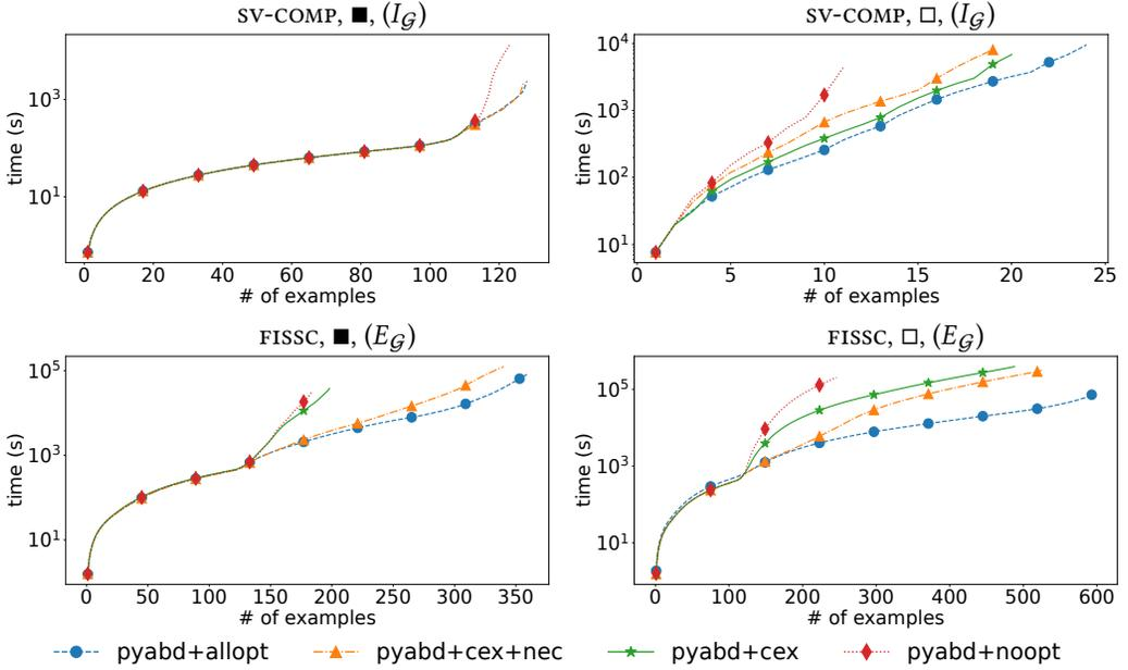
Fig. 5. Cactus plot showing the influence of the strategies of Section 5 on the computation of the first sufficient  $k$ -reachability constraint with PyABD.
