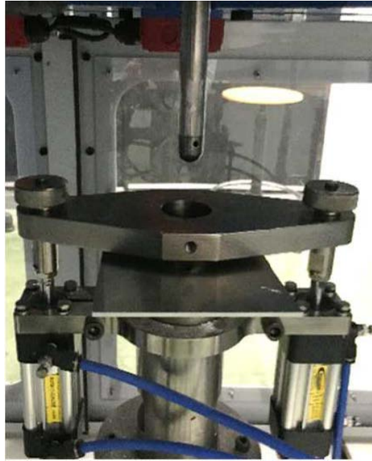
Figure 2. Impact testing setup showing a composite coupon clamped over the base supporting plate.
