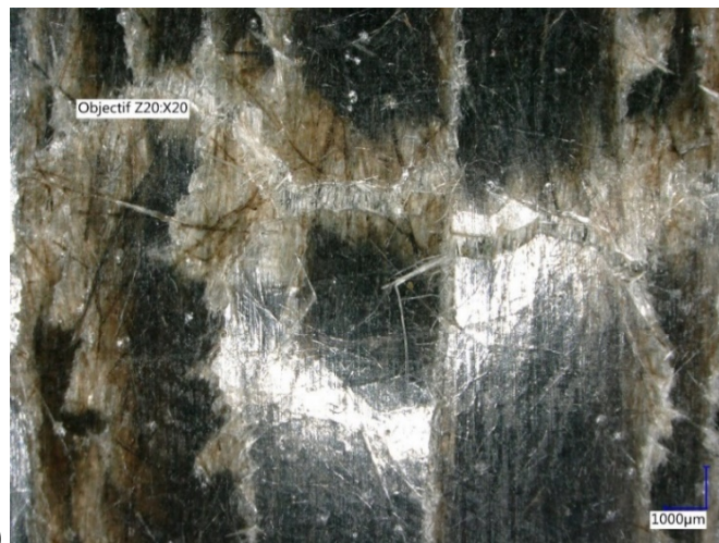
Figure 8. a) Typical force versus displacement curves for the UD and UD-mat composites for the 12 J tests and b) enlarged view of the back face of UD-mat coupon after impact at 12 J.
