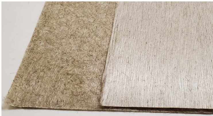
Figure 1. Typical UD flax-mat reinforcement used. The mat binder (left) and UD layer (right) are shown.
