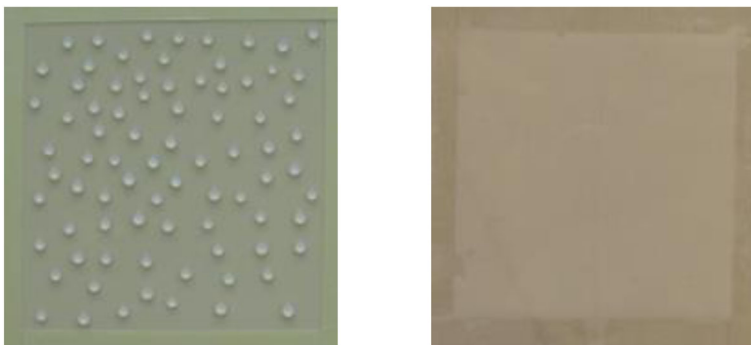
Fig. 3 Slab covered by a distribution of water drops (on the left) and by a uniform thin film (a surface of 80 cm 2 is delimited with a double-sided adhesive tape)
