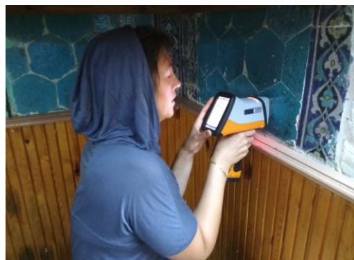
Figure 2. (a) Base-line subtracted representative Raman spectra showing different types of glazes (lead-rich, lead-alkali, and alkali-rich). The baseline has been subtracted in order to compare the bending to stretching band area ratio. (b) On-site measurement with pXRF in Edirne Şah Melek Paşa Mosque.
