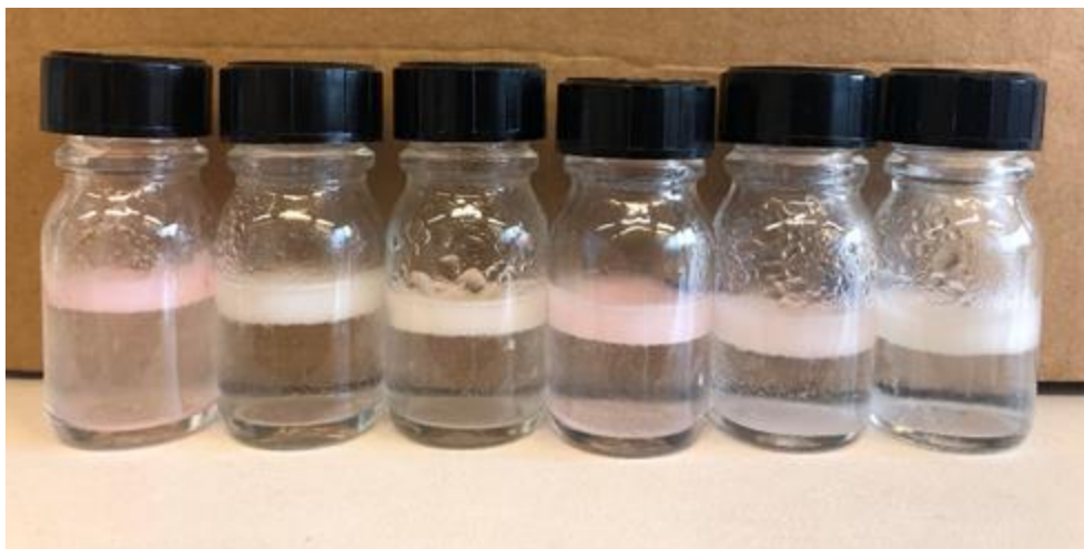
Figure S3. Pickering emulsions made with 25 mg of particles per cm 3 of oil. From left to right N-, A-, C-, A/N-, N/C- and A/C-emulsions. The picture was taken 4 months after the preparation of emulsions. No release of free oil was observed on top of the emulsions.
