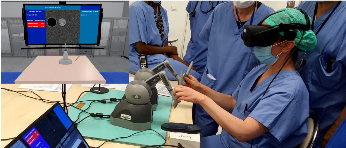
Figure 1: The user interface of UlTRASim including a head-mounted display with two tracking cameras to visualize the virtual scene and two haptic devices to control the virtual instruments. (Top left) The virtual scene as seen by the user with the virtual instruments manipulated by the user and the ultrasound screen displaying the ultrasound image.
