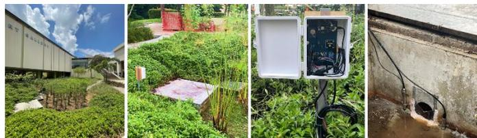
**Figure 8** Field implementation of the water level monitoring system in NIE rain garden in NTU, Singapore. One water level LCS, one water level TS and one temperature LCS were installed in the outlet sump.
