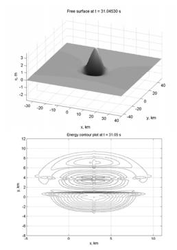
Figure 1. Free-surface snapshot and energy contour plot around the tsunami generation region. At t=31s.
